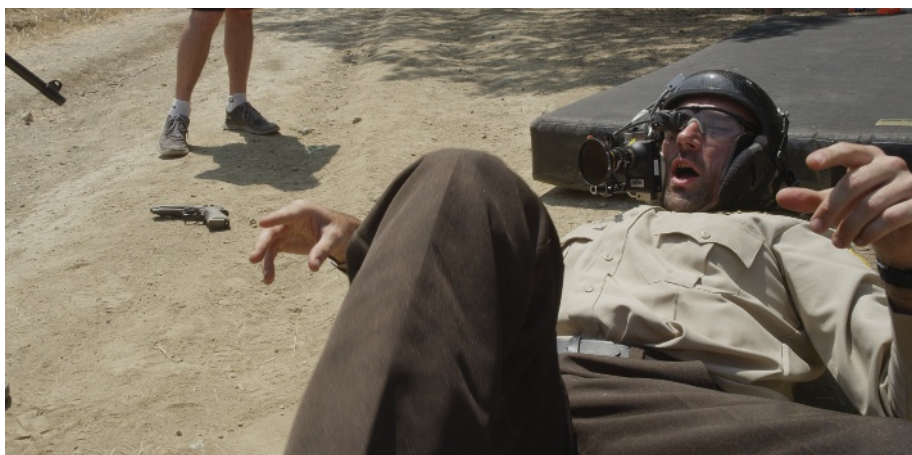
To simulate the police officer's perspective, Perkinson wore a customized helmet cam. Footage was recorded in 12-bit raw 2K to a Cinedeck Extreme HD bolted to a wearable backpack frame, and images were monitored via a Teradek Bolt wireless system.
